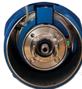
Source Assembly in secured position
