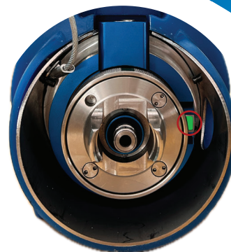
Source Assembly is in the secured position.
