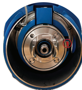
Source Assembly locking mechanism is released and ready to expose
