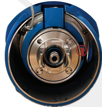
Source Assembly locking mechanism is released and ready to expose
