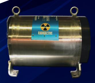
The signal indicator operates as follows: When the source is safely contained within the projector and the projector is locked in the «Safe» mode, a green signal is displayed. When the source is inside the projector but the projector is unlocked, and the source assembly locking mechanism is ready for release, a yellow signal is displayed. Lastly, when the source is either ready for exposure or outside the projector in the «exposure» mode, a red signal is displayed.
