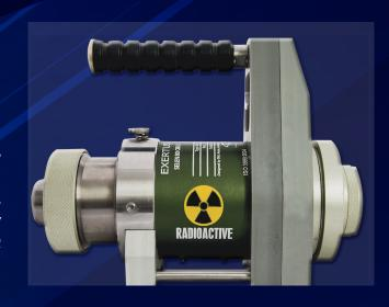
These projectors are capable of accommodating Selenium 75 sources. With its cutting-edge design, this projector offers a combination of flexibility and compactness. It can be utilized for both standard radiography techniques and situations that re-quire close proximity work.
