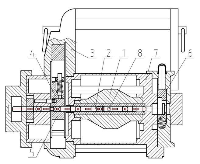
1 – Protection unit; 2 – Source holder; 3 – Flange; 4 – Fixing unit; 5 – Locking system; 6 - Locking system; 7 - Body; 8 - Source
